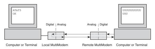
Figure C-3. Local digital loopback test.
